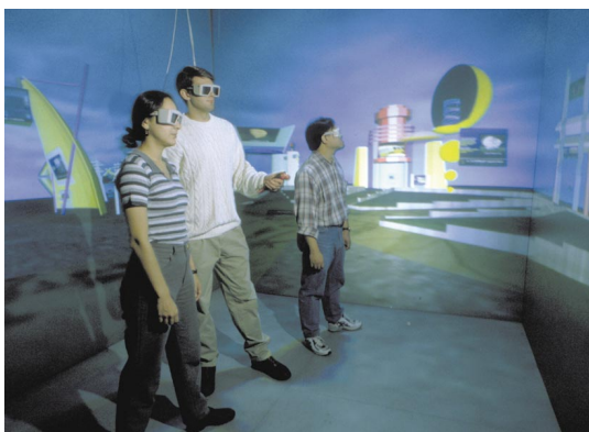
Figure 1. The CAVE (Cave Automated Virtual Environment). CRT projectors project stereoscopic computer images onto the CAVE's translucent walls, giving the occupant (user), who is wearing special glasses, the illusion that objects surround him. The user interacts with the environment through a wand (not shown). —Image courtesy of the Electronic Visualization Laboratory
