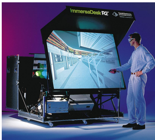
Figure 2. The ImmersaDesk. Like the CAVE, the ImmersaDesk projects stereoscopic images, but it is designed for images on a desktop scale, such as CAD models. —Image courtesy of the Electronic Visualization Laboratory
